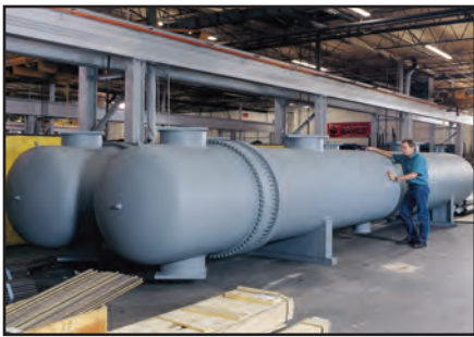
TEMA BEU Exchanger for Wastewater Treatment
